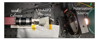
Polarization is generated in the lab by rotating a linear sheet polarizer in front of a diffuse light source. The HARP prism is then tested at each port and the results guide how to situate the final polarizers in front of the CCD camera yet to be placed. This test is necessary to ensure the quality of the antireflection and splitting coatings applied.
